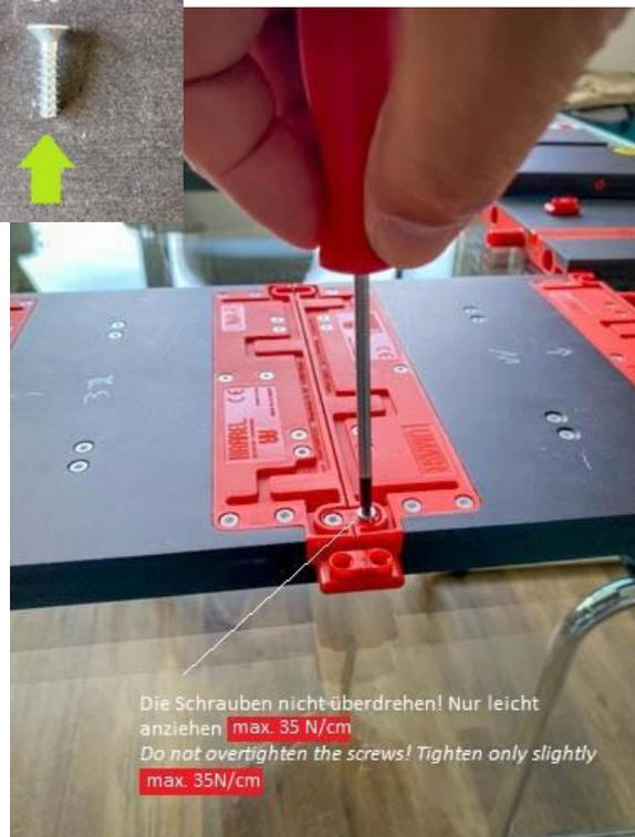
The inserted connectors are screwed together with the Harrel screw S-1 as pictured. This is done with the Harrel screwdriver STX-10 or a standard screwdriver with Torx-10 drive. When using an electric screwdriver, please make sure to observe the torque setting. Please tighten the screws only slightly (max. 35 N/cm).
